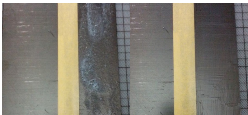
Figure 3. The Lithium Grease is applied on the non-abraded overlap area using a spatula.
