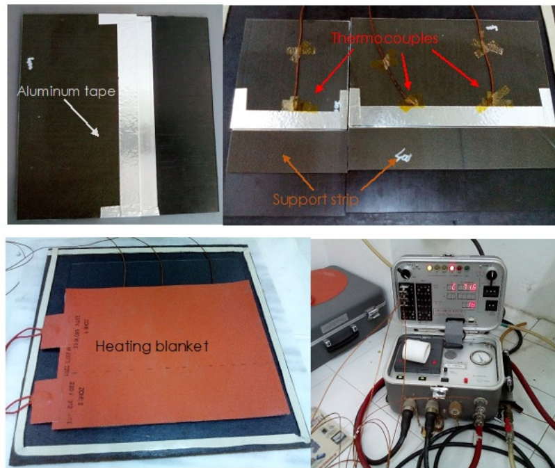
Figure 4. Out of autoclave curing using the hot bonder ANITA (GMI AERO) and a heating blanket
