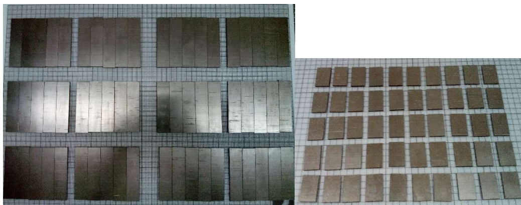
Figure 4. The joints (60) and tabs (50) that were cut from the composite panel
