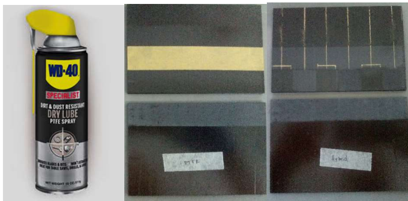
Figure 19. The PTFE lubricant is applied on the surface of the joint around the bonding area
